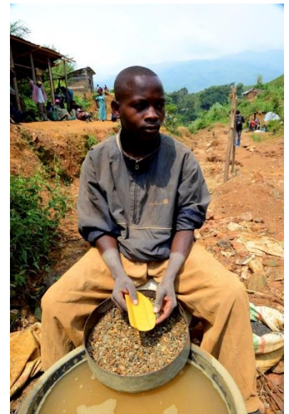
Below: A washer separates the tin ore.
